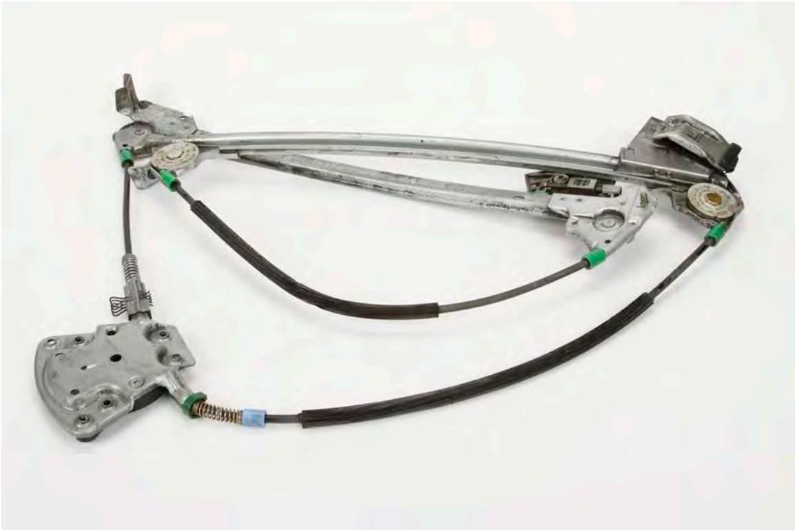
COMPLETE WINDOW REGULATOR WITH DAMAGED SLEEVE
