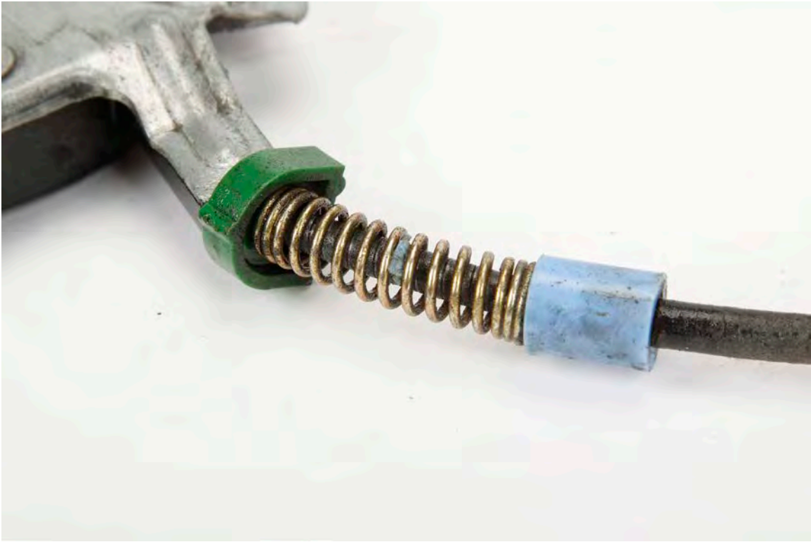
THE PLASTIC ORIGINAL FACTORY WINDOW REGULATOR SLEEVE THAT IS DAMAGED
