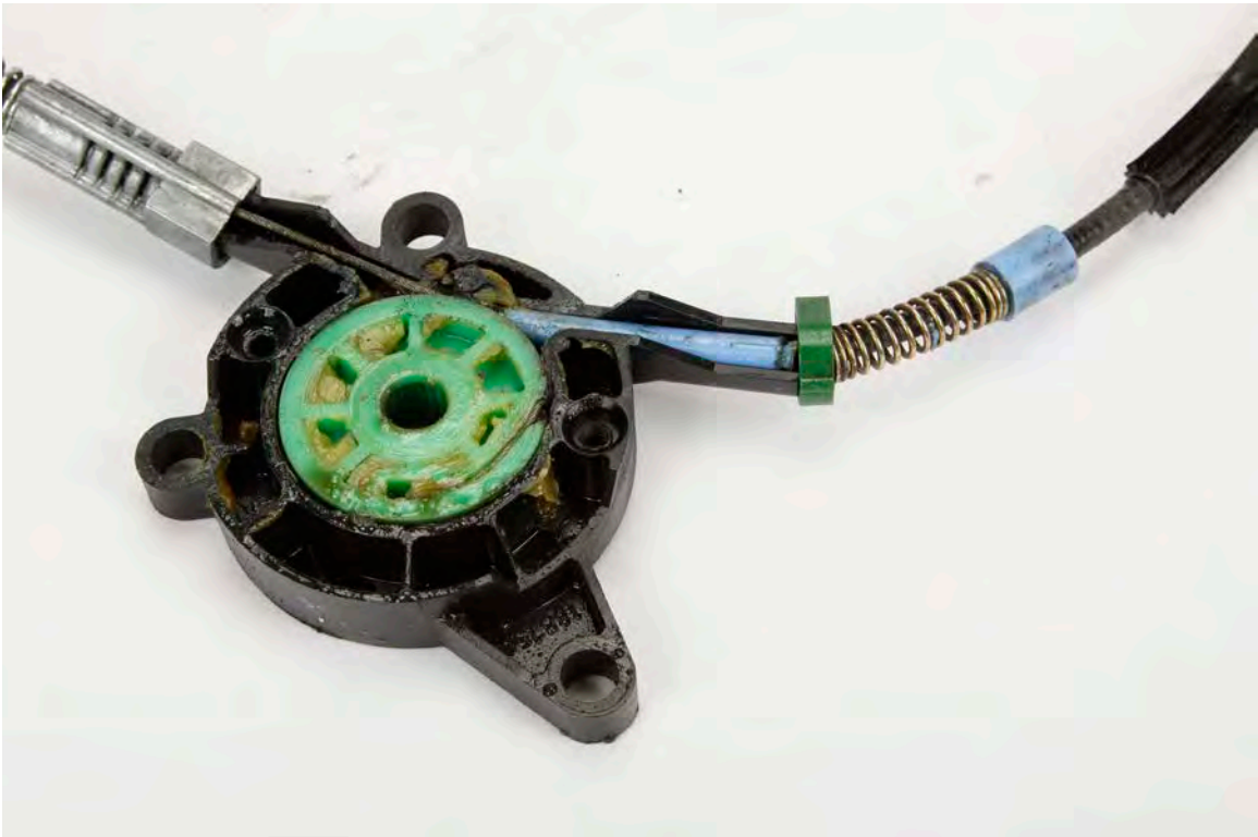
THE GEAR WHEEL WITH THE BROKEN OLD SLEEVE
